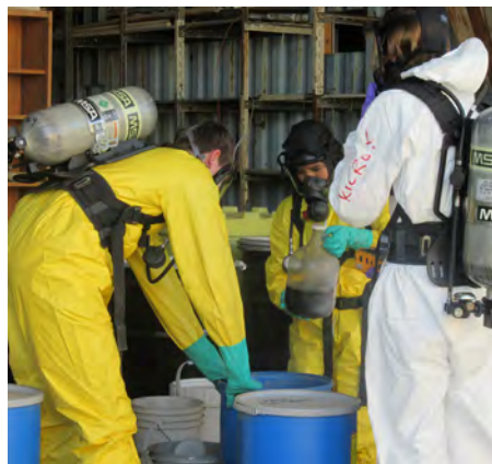
Toxic Substances Control staff wearing personal protective equipment check barrels of unknown chemicals/contaminants.
